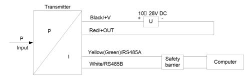
c) Wiring for HART®transmitter connecting with hand-communicator:
