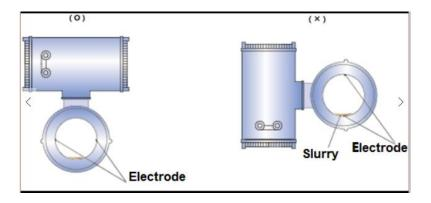
Electromagnetic flowmeter must work in full pipe conditions, that is to say, the flowmeter cannot work normally in partially filled pipe or empty pipe conditions.
